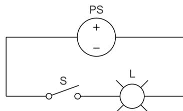
Figure 1. Schematic diagram of a circuit made of a power source and a switch controlling a lamp.
