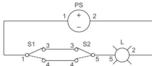
**Schematic diagram of a circuit made of a power source and two three-way switches controlling a lamp.**
